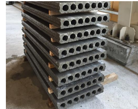
Hollow core slabs for walls and floors up to 120 mm high, 600 and 1200 mm wide (Nano Extruder System)
